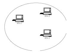
Figure 2-1 Ad Hoc wireless network
